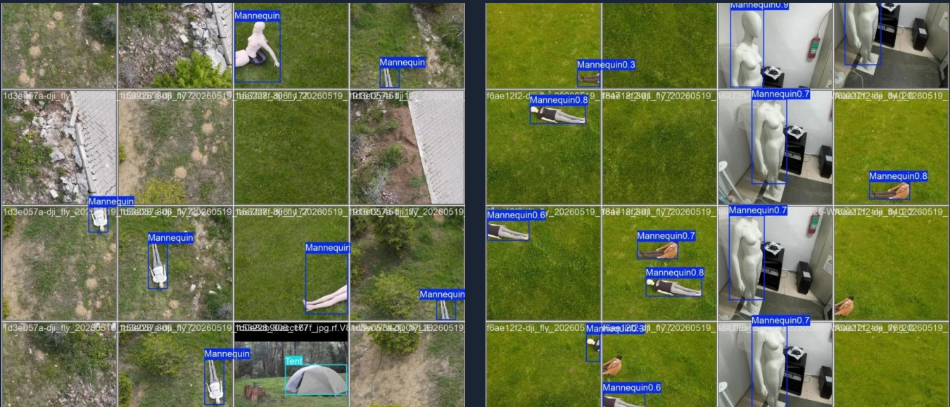
Validation output of the trained YOLOv11m model, with confidence scores across different altitudes, ground surfaces and lighting
