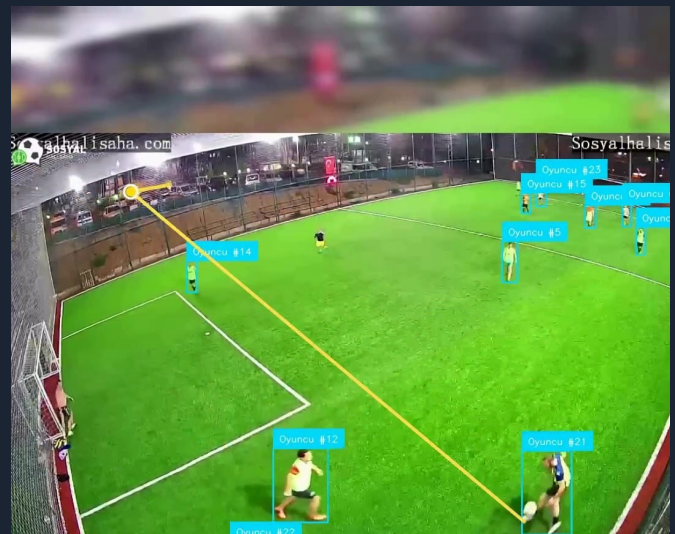
Ball trajectory tracking: linking positions across frames
